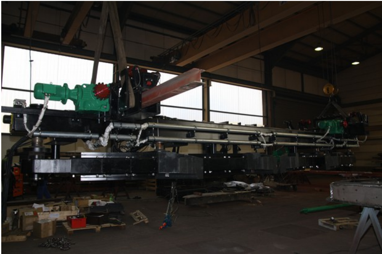
Picture 1: Drag plough feeder coke step 1 (overall length ~12m)
