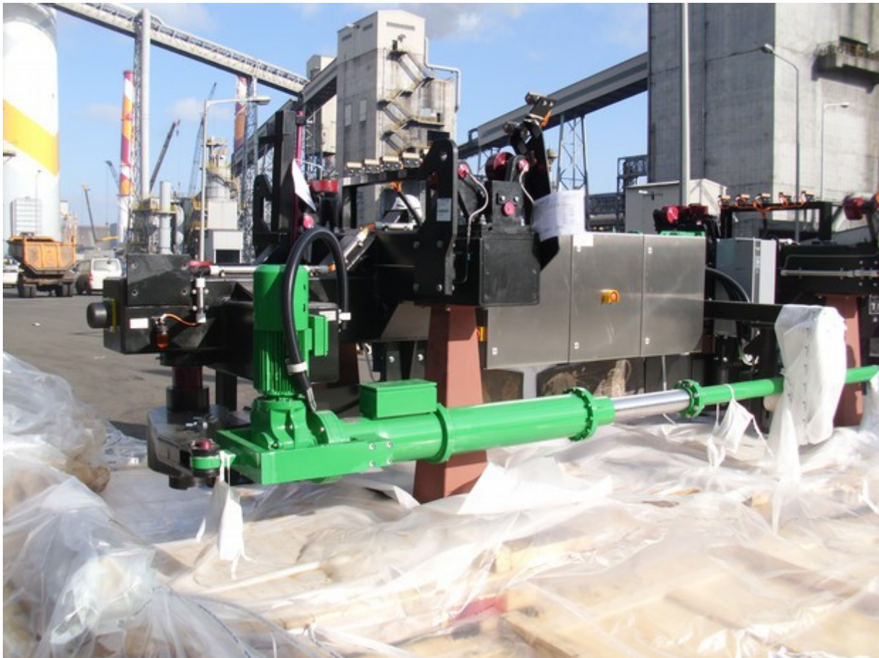
Picture 3: Drag plough feeder coke step 3 (transport completely assembled possible)
